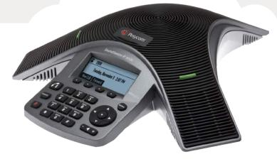
from up to 7 feet away. The phone also features technology that resists interference from mobile phones and other wireless devices, delivering clear communications without distractions.
